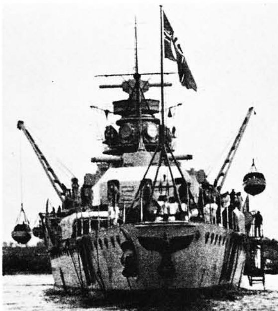
A further point of difference: in contrast to the Admiral Scheer, the Graf Spee had heavy loading gear on both sides (the Scheer only on the port side).
