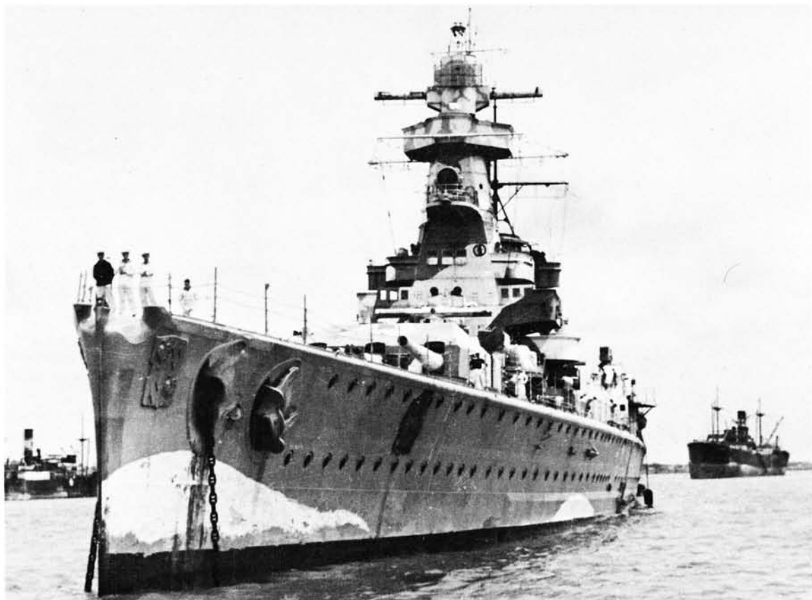
Admiral Graf Spee at Montevideo after the battle. The hole from a direct hit on the port bow has been plated over by the ship's staff
