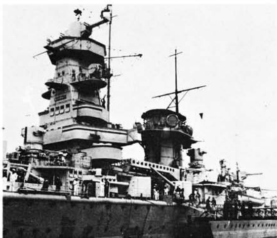
The Graf Spee differed from her sister-ship the Admiral Scheer in having, behind the tower-mast, a pole-mast rising from the signal-deck level (the Scheer only had a short pole-mast on the foretop gallery), and further in having her mainmast supported by short support-legs to the funnel. The conspicuous tower-mast was completely rebuilt on the Scheer in the light of the Graf Spee's experience.
